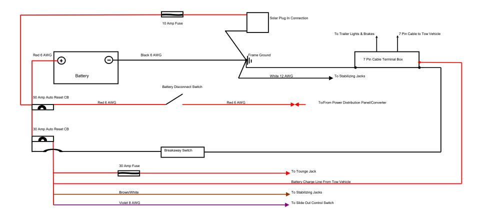
Battery Disconnect Switch disconnects all DC to trailer except for stabilizing jacks, slide out, tounge jack.
