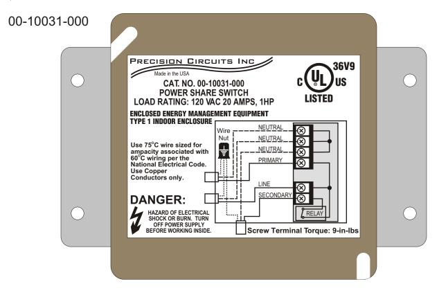
Power Share Switch (PSS) provides the capability to wire two appliances to a single circuit breaker. The Primary appliance never losses power. The Secondary appliance is allowed to run as long as the Primary is not drawing current. Power to the Secondary appliance is turned off whenever the Primary Appliance is drawing current.
