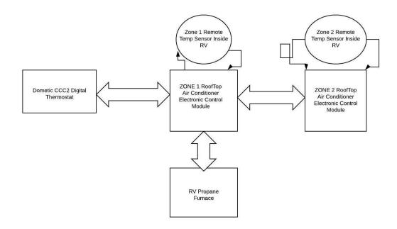
Flow of how the Dometic CCC2 Digital thermostat communcates back and forth to the Zone 1 and Zone 2 Air conditioner units, Heat Pump on Zone 1, Furnace, and remote temperature sensors for both Zone 1 and Zone 2 located inside your Alpine. DATA commands are sent across the CANBUS on 2 wires from the RJ45 telephone cable connections from the CCC2 Thermostat, up to the Zone 1 and Zone 2 AC Unit electronic control modules.
