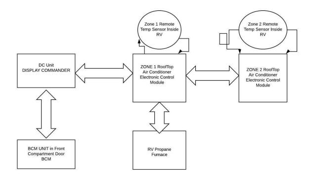
Flow of how the IN Command system communcates back and forth to the Zone 1 and Zone 2 Air conditioner units, Heat Pump on Zone 1, Furnace, and remote temperature sensors for both Zone 1 and Zone 2 located inside your Alpine. DATA commands are sent across the CANBUS on 2 wires from the RJ45 telephone cable connections from the DC to BCM, up to the ZOne 1 and Zone 2 AC Unit electronic control modules.
