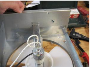
Attach the duct piece to the back of the hood with pop rivets.
