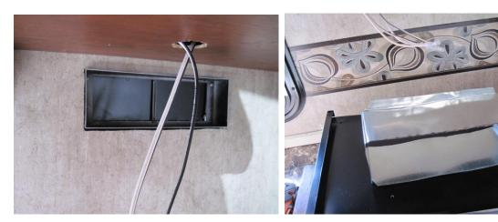
Once you are certain all parts are ready for installation, line the vent edges with butyl tape. Place the vent in the opening and secure with stainless steel screws. Carefully trim excess butyl with a hobby knife. I later sealed vent with RV sealant.
