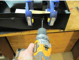
After drilling out the welds remove the metal plate. You may have to use a chisel to break the welds free.
